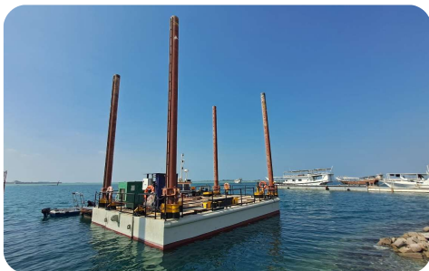
GEOTECHNICAL INVESTIGATION USING MODULAR PONTOON AND SPECIALIZED MARINE EQUIPMENT
